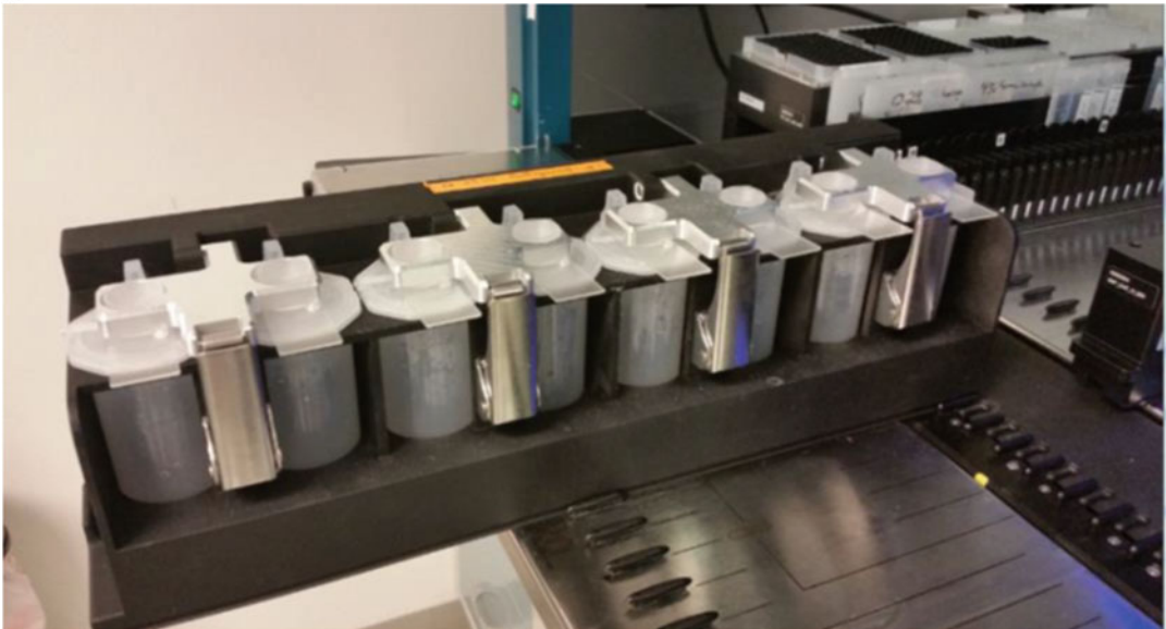
Fig. 1 The filtration system. (a) Design of the microfluidic filter device and the schematic overview of the processing steps for capture and detection of circulating rare cells. The filter membrane is mounted onto microscope plastic slide with microfluidic structures. The top of the membrane is exposed to the pipetting system of the robot, while the underside of the membrane is welded on the outer ring of the plastic support and is contact with the microfluidic structures. The structure consists of microfluidic posts, which allow for controlled filtration across a pressure range of negative 10–30 mbar as well as efficient washing of cells during the isolation and staining process (reproduced from Magbanua et al. 2015 [8]). (b) The disposable microscope plastic slide is integrated into a waste container with a top well for holding 5 mL of liquid and a bottom waste container capable of holding 110 mL of waste liquid. The waste container encloses around the top and bottom of the slide when mounting onto the filtration unit. The waste container connects directly to the vacuum from the underside of the slide
