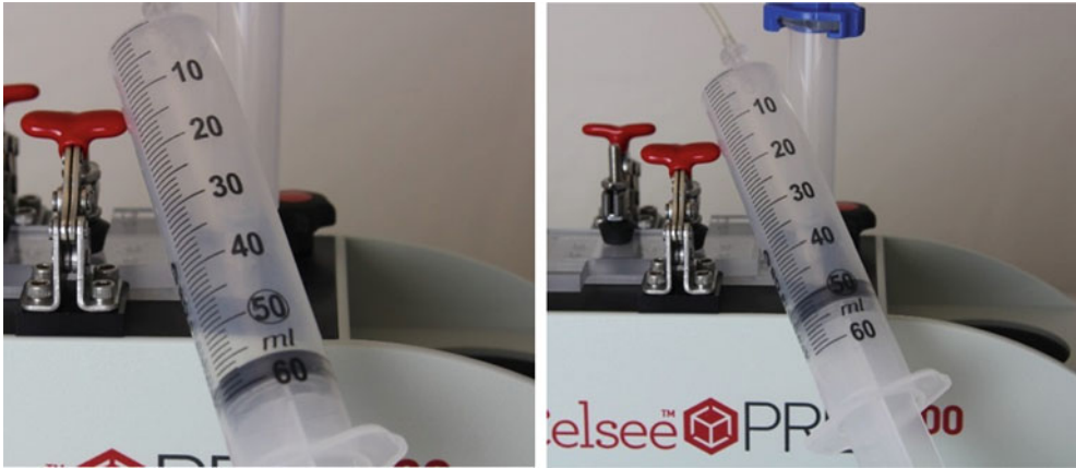
Fig. 4 Pulsing procedure to backflow cells from the microfluidic slide for cell enrichment and retrieval
